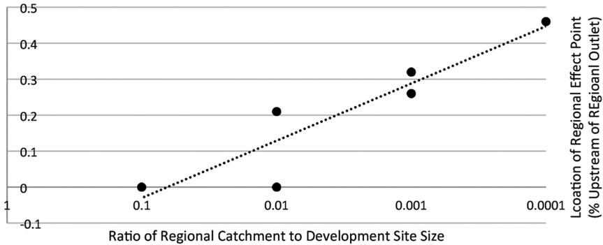
**Figure 6** – Location of Regional Effect Point relative to catchment size, based on the results from six catchments used in this case study.
