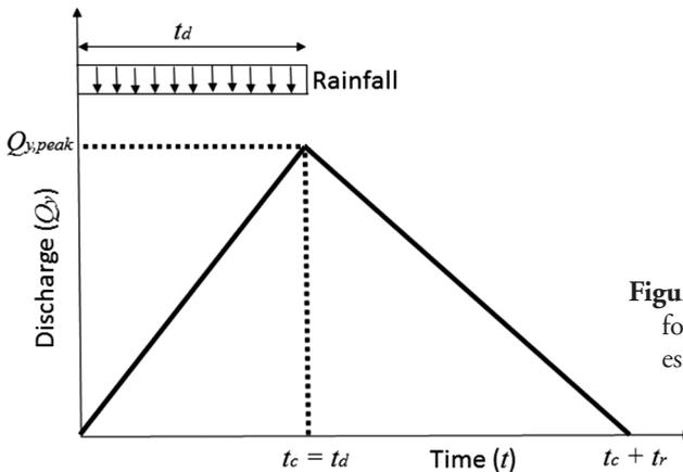
Figure 8 – Triangular method for storm hydrograph estimation.
