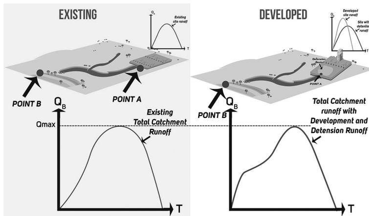
**Figure 2** – The total catchment approach to stormwater detention design.
