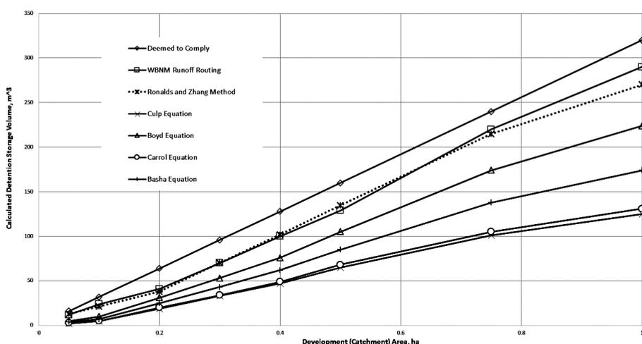
**Figure 11** – Comparison of stormwater detention storage volume results derived from various methods.
