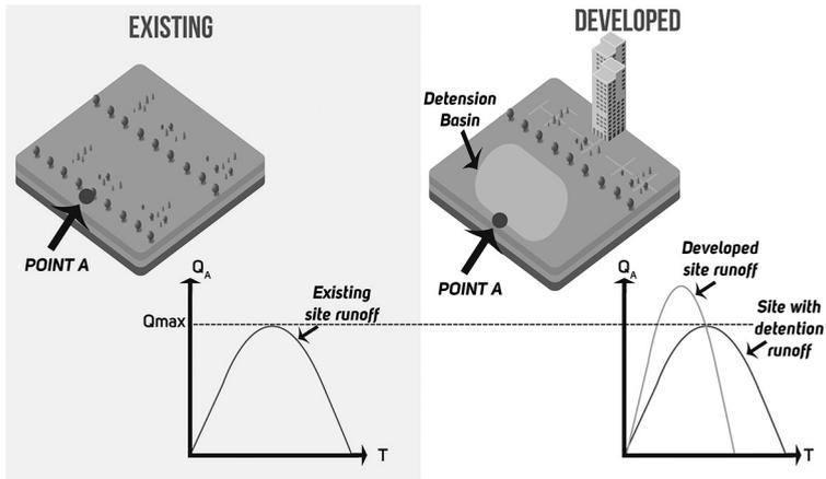
**Figure 1** – The micro-management approach to stormwater detention design.
