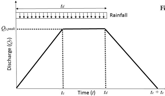
**Figure 9** – Trapezoidal method for hydrograph estimation.
