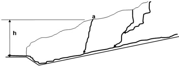
**Figure 2** – The maximum pressure difference over the lower reach of the conduit system is  $h$ . Any greater pressure difference would cause water to back up and spill out of moulin  $a$ .
