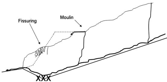
**Figure 4** – Piezometric pressure (dotted line) in subglacial conduit system with partial blockage (XXX) in lowest point of system causing high longitudinal pressure gradient.
