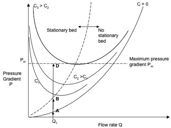
**Figure 1** – Pressure gradient  $P$  vs water flow rate  $Q$  for gravity-driven flow in a pipe with various sediment concentrations  $C$ .
