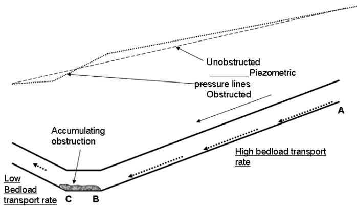
**Figure 3** – Sediment accumulation in a conduit reach of decreasing or reversing slope.
