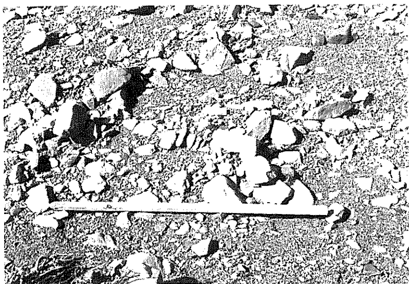
FIG. 3—Example of the type of particle cluster that occurs widely on the bed of the Kowai in the study reach. Flow was left to right. Stake is 1 m long.
