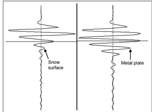
**Figure 3** – ‘Wiggle’ trace obtained from the air-coupled 800 MHz antenna suspended over the snow surface alongside the trace obtained from the antenna in the same configuration over a metal plate on the snow surface; the traces have not been filtered.
