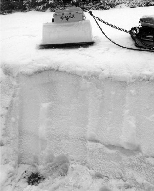
**Figure 2** – A snow bank that is about 1 m high with 800 MHz GPR antenna shown in air-coupled configuration, sitting on an upturned plastic box some 270 mm above a 2-mm thick, 0.6 m × 0.6 m metal plate, resting upon the snow surface.
