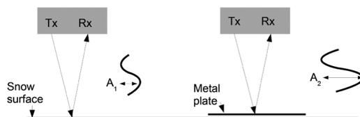
**Figure 1** – The surface reflection method compares the amplitude of reflection from the medium surface ( $A_1$ ) with that from an assumed ideal reflector (metal plate) ( $A_2$ ).
