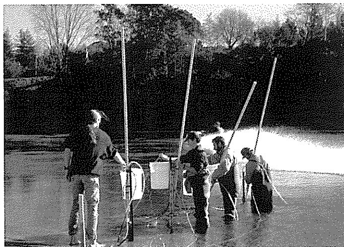
Figure 3 – Wave measurements and suspended-sediment samples were collected at each sensor position under a wide range of conditions.
