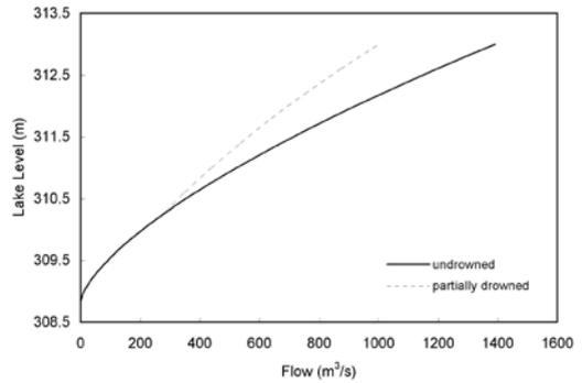
**Figure 9** – Effect of partial drowning of the Lake Wakatipu outlet on the weir discharge rating, based on an assumed tailwater rating curve.
