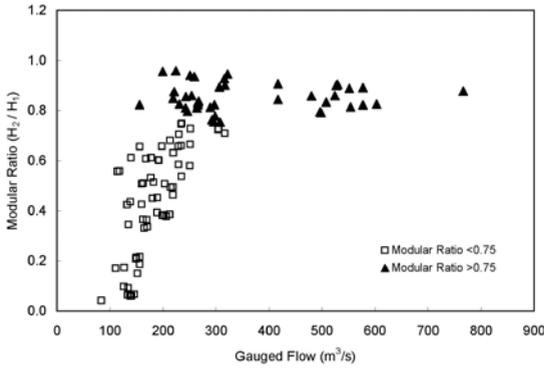
**Figure 6** – Modular ratio as a function of gauged flow for the Lake Wakatipu outlet weir.
