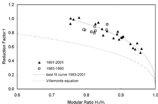
**Figure 8** – Flow reduction relationship for the Lake Wakatipu outlet weir under partially drowned conditions.
