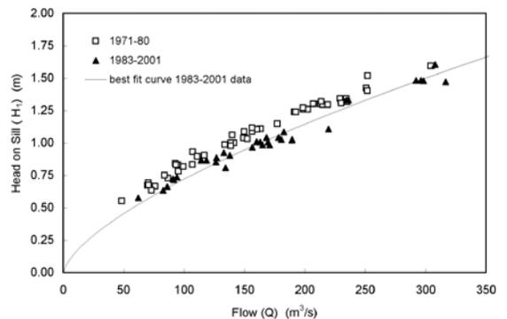
**Figure 7** – Discharge rating for the Lake Wakatipu outlet weir under free discharge conditions.
