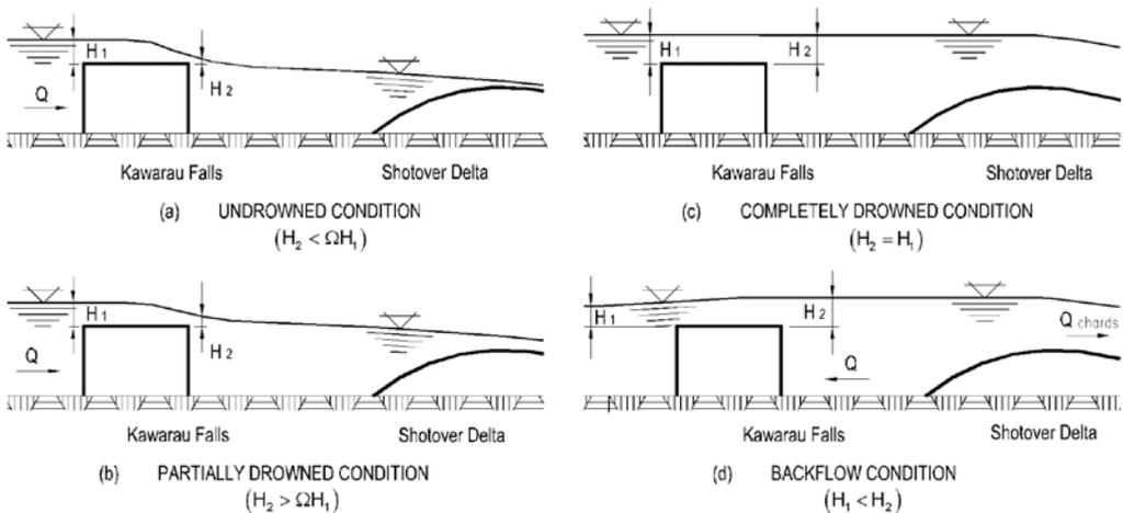
**Figure 5** – Flow out of Lake Wakatipu under (a) undrowned (free discharge), (b) partially drowned, (c) fully drowned and (d) reverse flow conditions.
