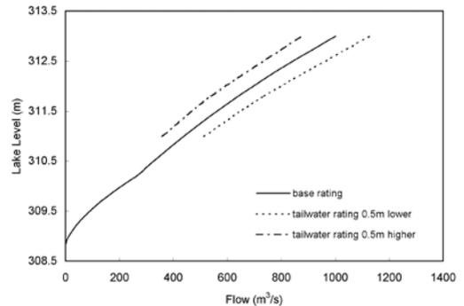
**Figure 10** – Discharge rating for the Lake Wakatipu outlet weir for variable tailwater level conditions.
