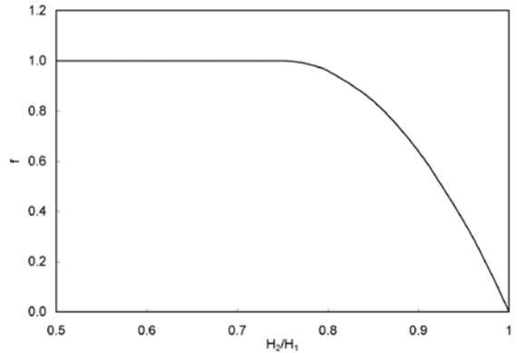
**Figure 4** – Typical reduction factor curve for a partially drowned weir
