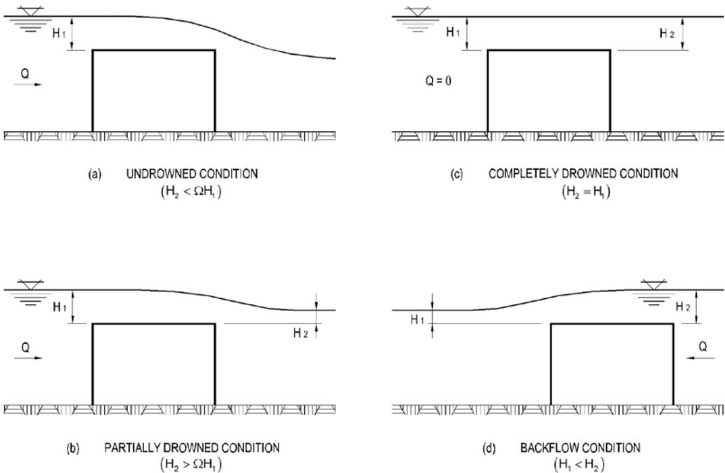
**Figure 3** – Flow over a broad-crested weir under (a) undrowned (free discharge), (b) partially drowned, (c) fully drowned and (d) reverse flow conditions.
