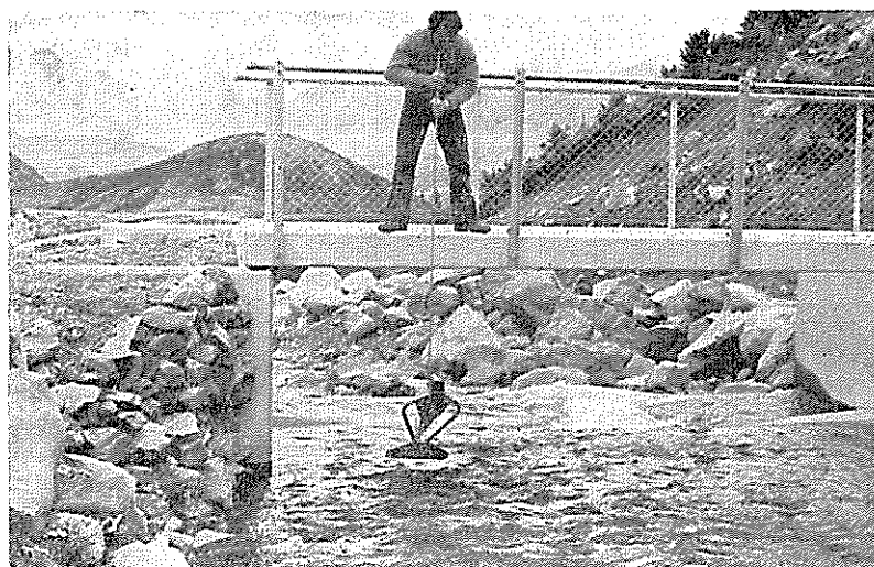
PLATE 1—View from upstream of operation of Helley-Smith Bedload Sampler from bridge across weir, Dry Acheron Stream, New Zealand.
