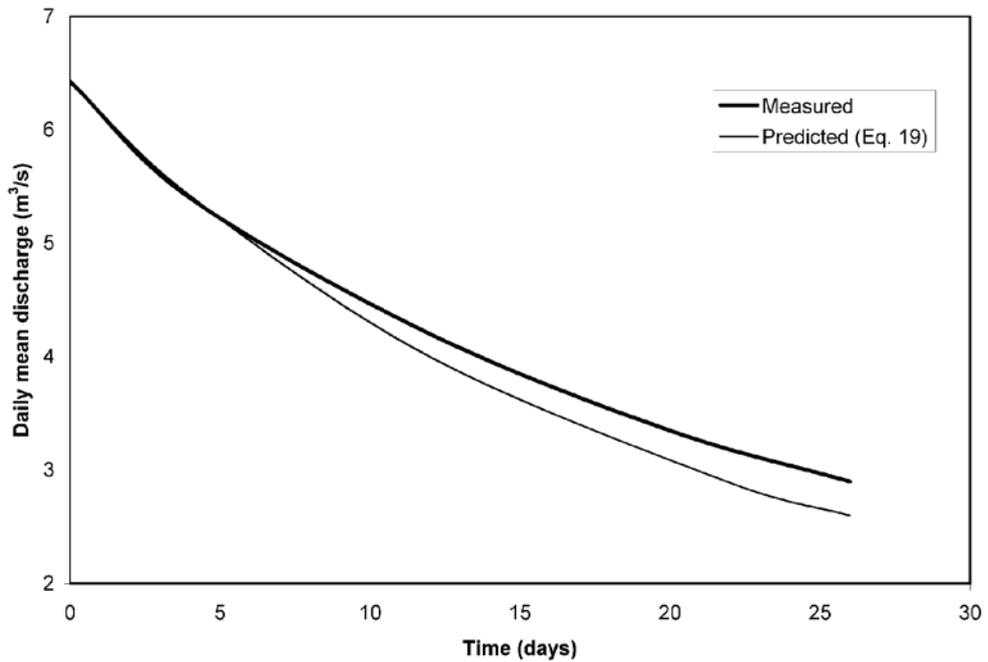
**Figure 2** – Predicted and measured baseflow recession curves for Jollie at Mt Cook Station (Site no. 71135).
