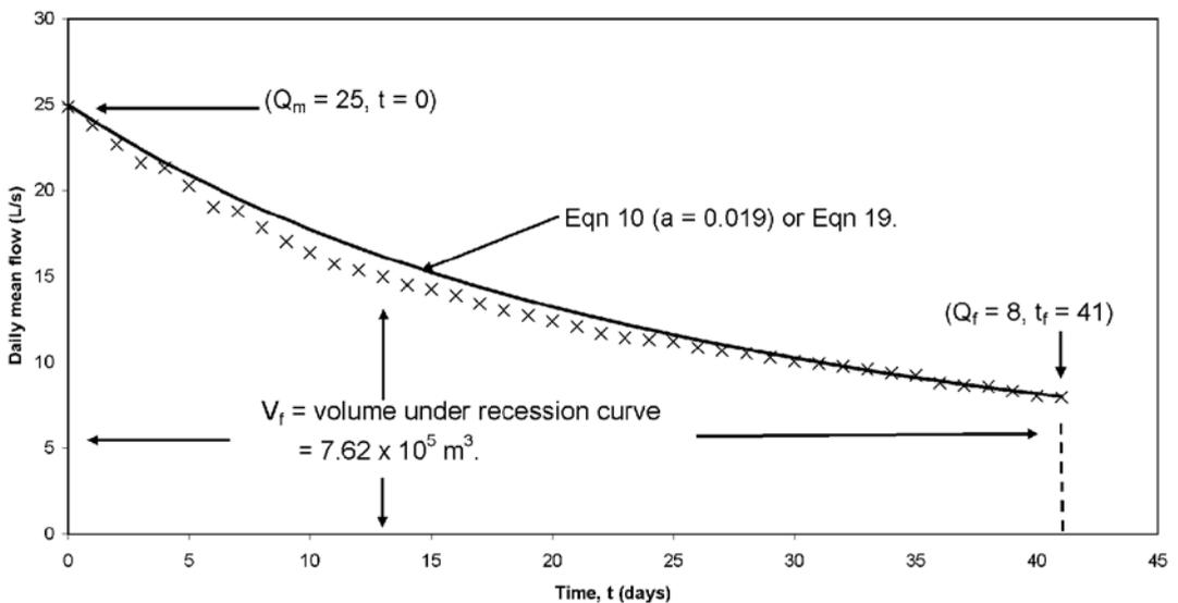
**Figure 1** – Master recession curve (x) for Camp Stream at Craigieburn (Table 1) and fitted recession curve (Eq. 19) showing definitions of variables.
