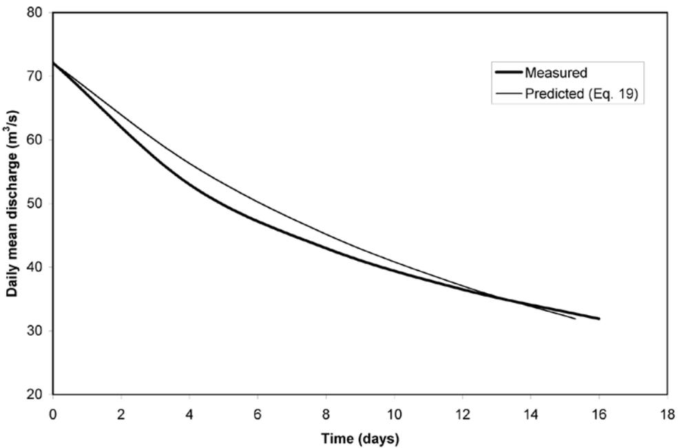
**Figure 3** – Predicted and measured master baseflow recession curves for Waiiau River at Marble point (Site No. 64602).
