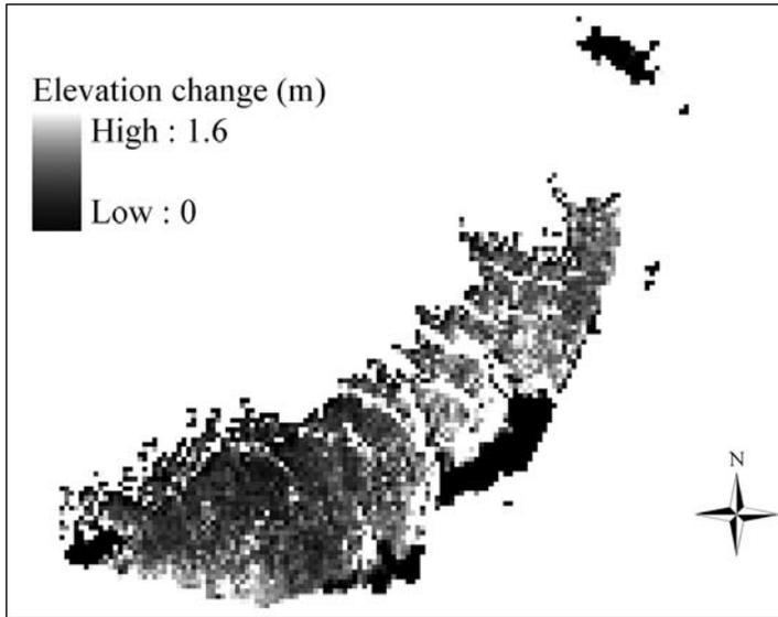
**Figure 4** – Vertical difference in surface elevation between 14 April and 13 March 2008 for that part of the glacier that was scanned on both occasions.
