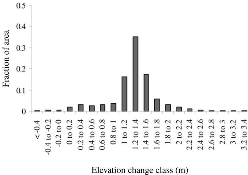
**Figure 5** – Frequency distribution of elevation change between 14 April and 13 March 2008 for that part of the glacier that was scanned on both occasions.
