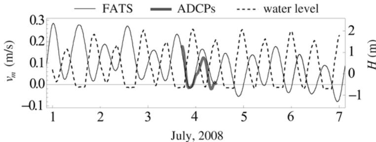
**Figure 4** – Comparison of cross-sectional mean velocity between the fluvial acoustic tomography system (FATS) and acoustic Doppler current profilers (ADCPs).
