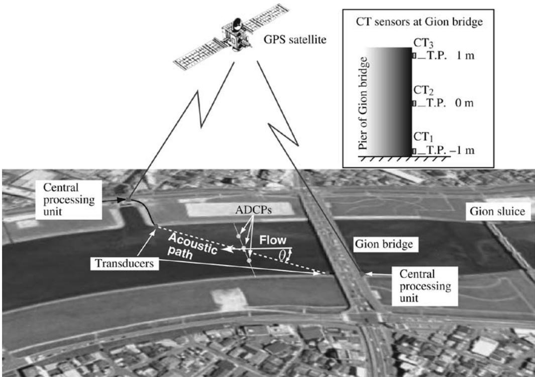
**Figure 2** – Schematic diagram of the method of measurement.
