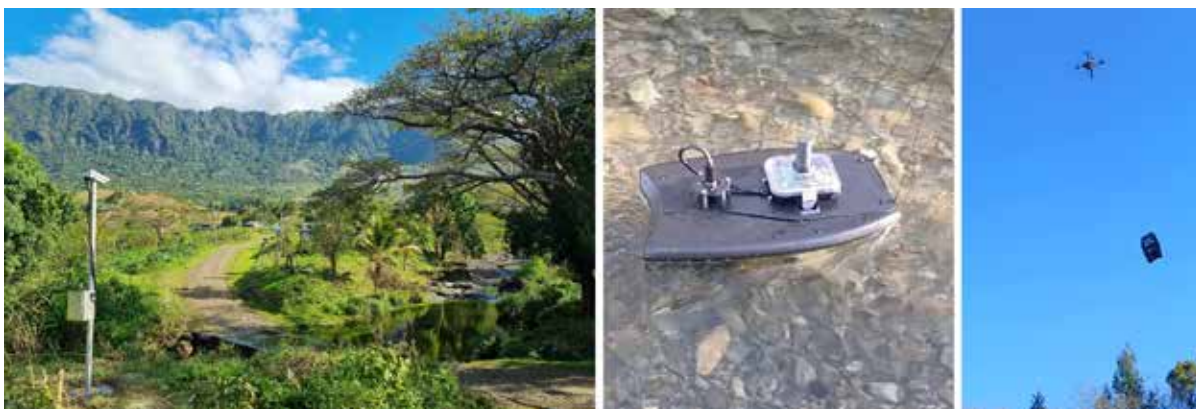
Figure 1: Stereoscopic camera station deployment in Fiji at a remote gauging site where access is cutoff during floods (left). Drone towed echosounder boat, with RTK GPS for origin and IMU for orientation (right).
