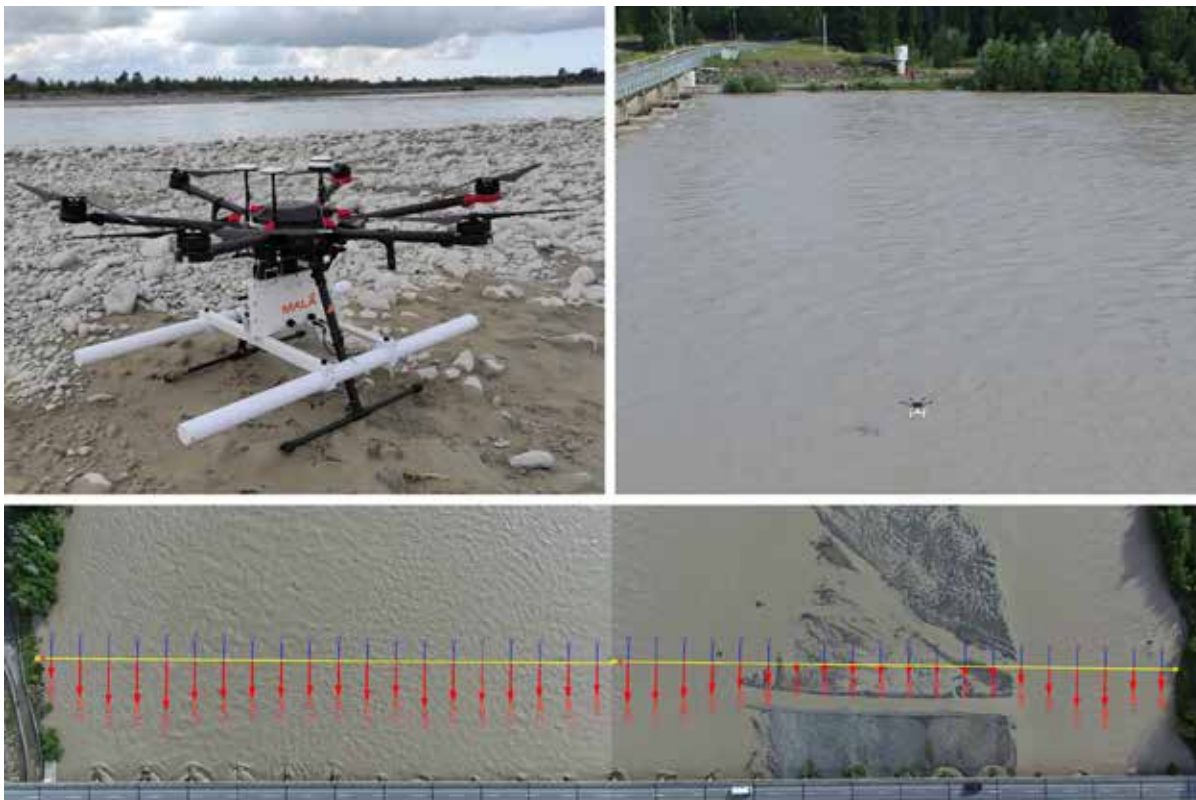
Figure 2: MALÅ GeoDrone 80 aerial Ground Penetrating Radar (GPR) system (top left) for flood cross section measurements (top right). Surface velocity measurements in sections in the Waimakariri River (bottom).
