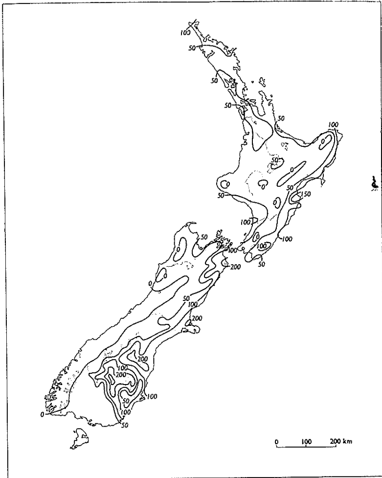
FIG. 1— Average annual water deficit ( DE ) in mm. (Deficiency of rainfall plus available soil moisture with respect to average Thornthwaite potential evapotranspiration PE , for soil moisture capacity S of 75 mm, based on a daily water balance.)
