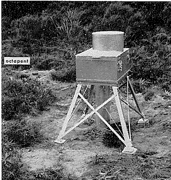
FIG. 4 — Casella 95-day automatic rain gauge and 27-inch octapent storage rain gauge at Makahu Saddle (3,200 ft).
