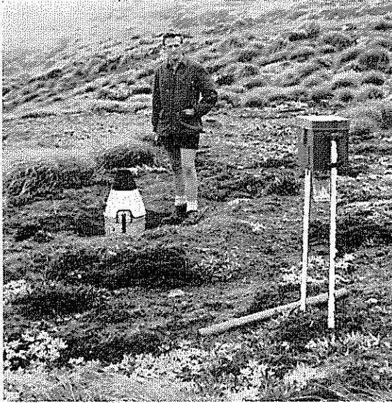
FIG. 5 — Type-C storage rain gauge and weatherproof stationery cabinet at Kaweka Trig (5,620 ft).
