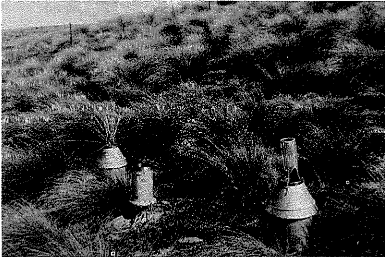
FIG. 2— Recording raingauges at the study site to compare catches of a fog interceptor (right) and 32 mounted snow tussock tillers (left) with that of a conventional gauge. April 1970.
